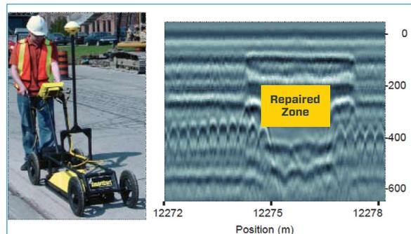
Assess the interior of concrete and pavement for asset management and maintenance planning.
